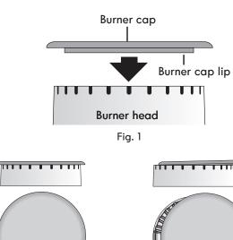
Correct burner cap placement
